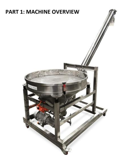
Flamingo auger conveyor is a powerful machine that can transfer powder/granule product from its product hopper onto the adjustable-height outlet.
