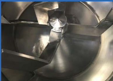
Internal wipers- Teflon / Metal detectable material
