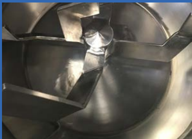
Internal wipers- Teflon / Metal detectable material
